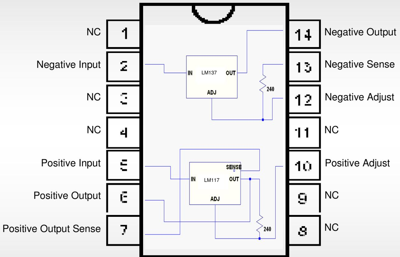
Electrically isolated adjustable positive and negative voltage regulators residing in a single package.
